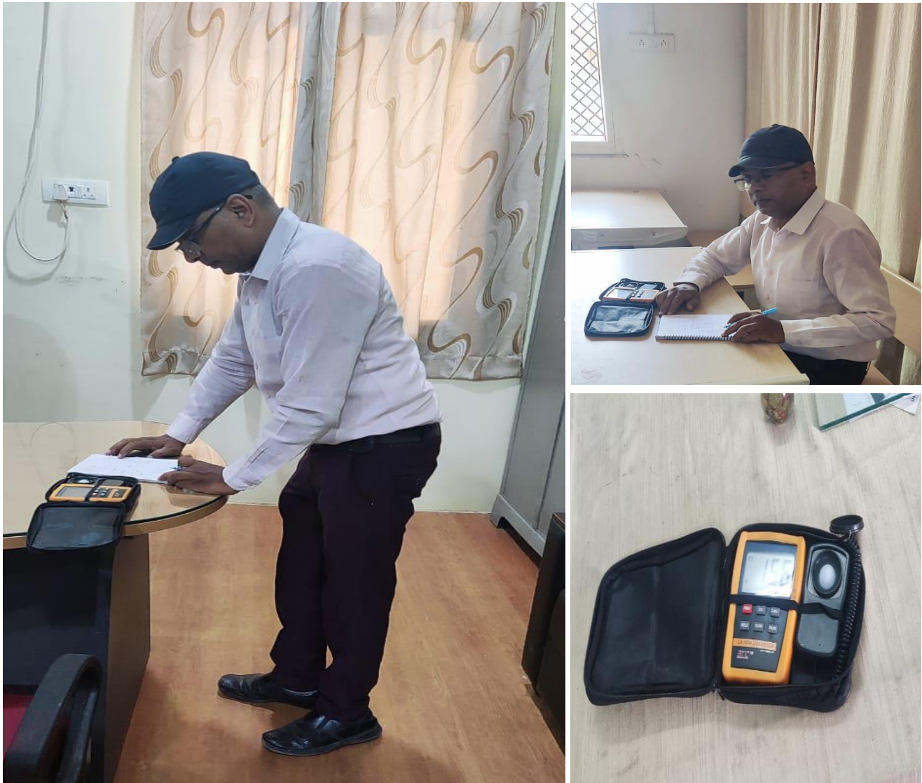
Figure 8 Lux Measurement at Site.
